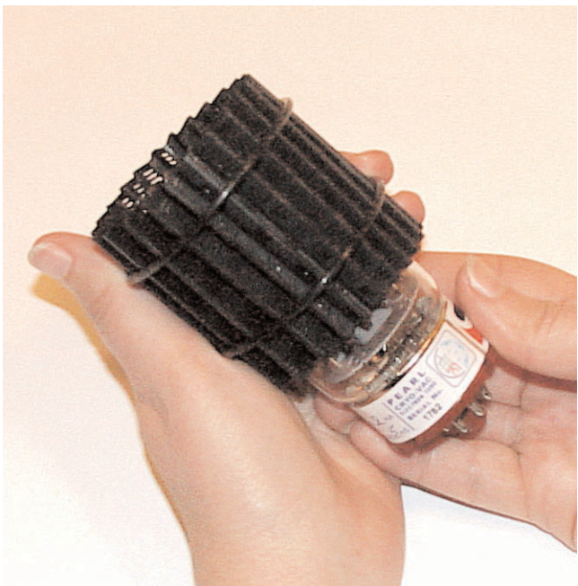
Fig. 4. Here, the cooler and sleeve combination can be seen properly fitting onto the tube.
