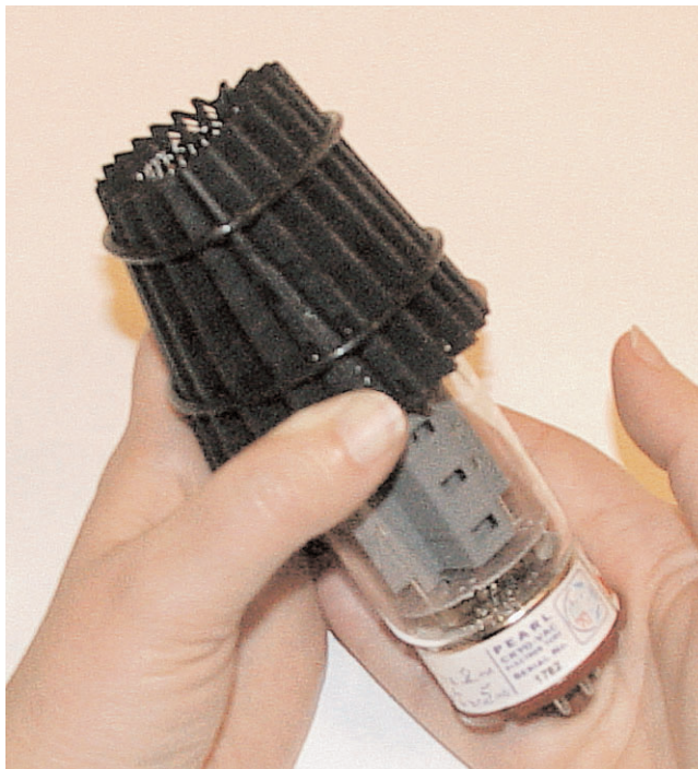
Fig. 3. Start the tube into the sleeve first, being sure not to push it out of the cooler. If necessary put a finger at its top end . . .
