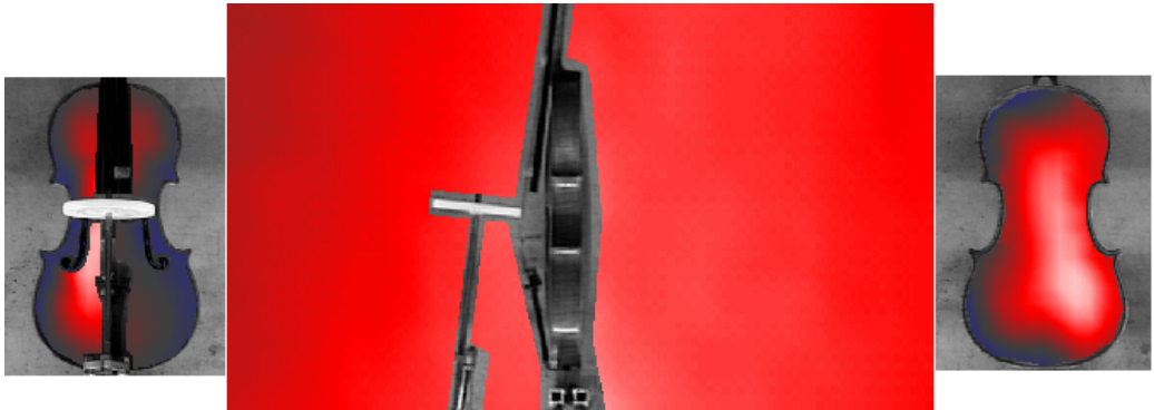
Figure 9. Vibration and sound fields at the first harmonic (285 Hz). (a) Top plate ODS, (b) sound field and (c) back plate ODS.
