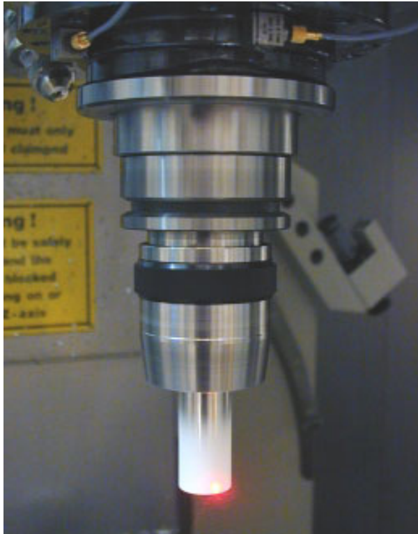
Figure 1. LDV measurement of the rotating optically raw (sprayed) dummy tool.
