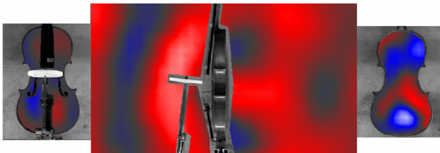
Figure 3.17: LDV measurements on a bowed violin and the generated sound at 1130 Hz, the fourth harmonic of the played tone.
