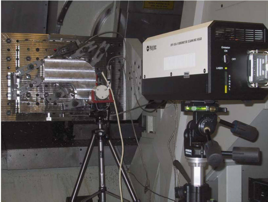
Figure 8. Photo of the setup with the stock and the shaker mounted in the Liechti machine.
