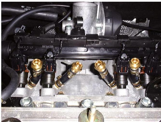
The length of the LPG hose between the SGI vaporiser and the Fuel Rail is not really important for the performance of the system (it is a good starting point to keep it as short as possible).
