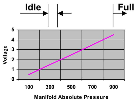
① When the SGI system is used in engines equipped with boost pressure (turbo), the reach of the MAP sensor integrated into the Interface Unit is not sufficient. In that case the original MAP sensor of the engine concerned must be branched off. In case the engine-management system is not fitted with a MAP sensor, a separate MAP sensor will be included in the SGI engine kit. Both situations are clearly explained in this installation manual.
