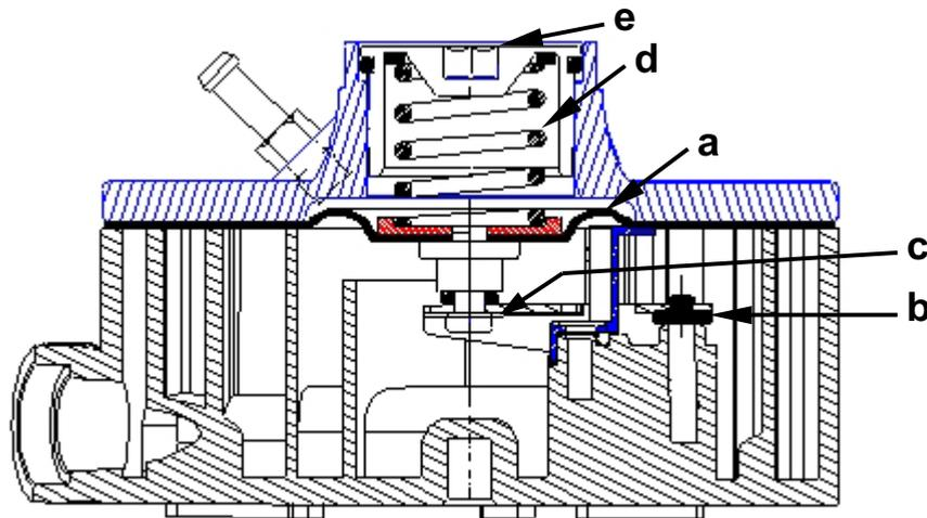
As shown, underneath the membrane (a) LPG is allowed to enter the vaporiser along the valve (b), which is fitted onto the lever (c); when the shut-off valve is open.
