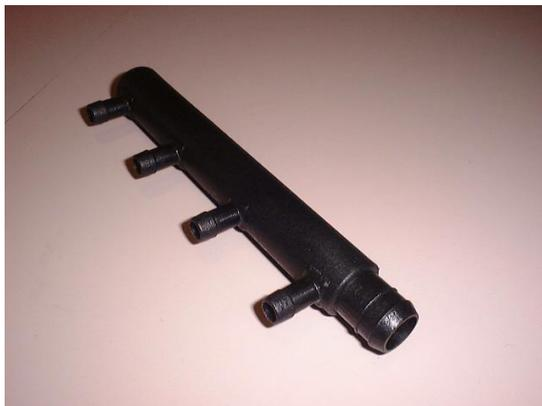
The fuel rail has the same function as the fuel gallery in multi-point petrol engines i.e. it only regulates the distribution of the LPG supply from the vaporiser to the SGI injectors. In addition to the present 4-splitter rail (AG 600.090), various versions will become available for 5- and 6-cylinder engines when required (8-cylinder engines are fitted with two 4-splitter rails).
