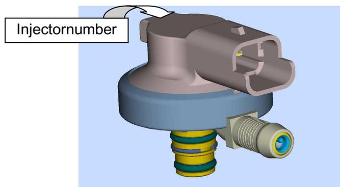
The operation of the injectors is based on a diaphragm instead of a plunger principle. Two conditions are possible:
