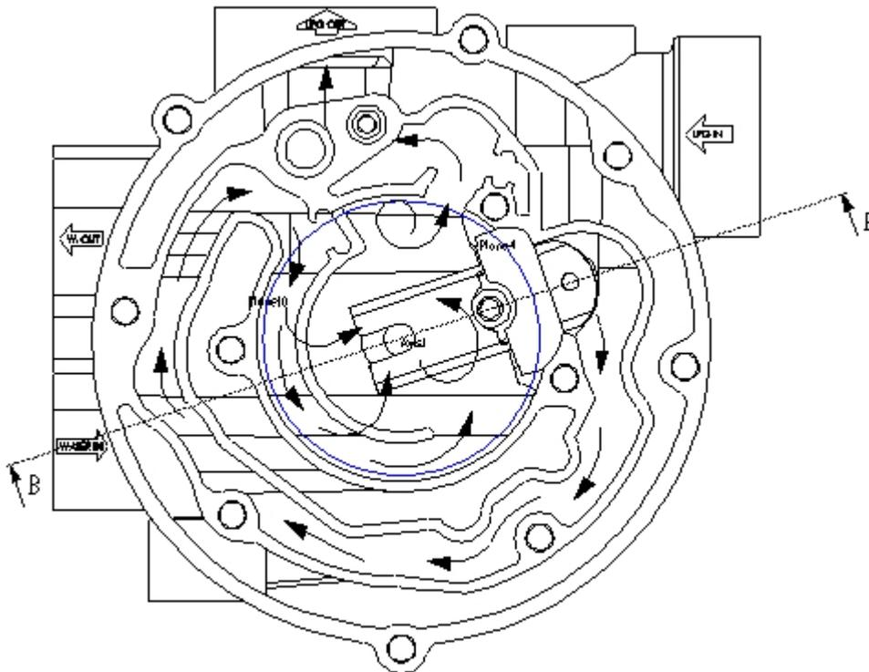
As shown above by the arrows, the velocity of the LPG is kept as high as possible during which the heat exchange in between the engine coolant and the LPG is optimal.
