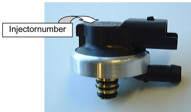
In case this number does not correspond to the part number referred to, the opening period of the petrol injector will not be converted exactly. The engine-management computer will have to correct the mixture to such an extent that this may cause problems, such as hesitation, stalling and the computer becoming deranged (check engine).
