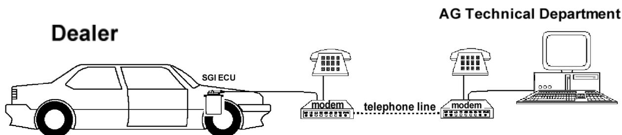
When all the necessary connections have been made, the switch should be set to LPG and the ignition off. Then the so-called modem line (see appendix) can be contacted, using the telephone in the test kit.
